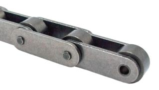
Large Roller Double Pitch, Straight Sidebar Chains, feature similar benefits to the standard roller series; however, their oversized roller projects above and below the sidebars to produce a rolling rather than a sliding action. They minimize friction across the supporting surface to reduce wear and power requirements in heavier-duty applications. These chains are indicated by adding "C" and 2002 to the ANSI standard chain number (e.g., C2062H).
