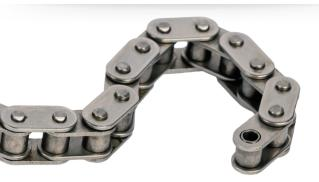
Standard Pitch Straight Sidebar Roller Chains dimensionally align with ANSI standards, except they substitute a straight-edged side plate for the standard "figure-eight" used for drive chains. This design is better suited to support and carry goods consistently. These chains weigh marginally more than standard roller chains and offer slightly increased fatigue strength. A "C" added to the corresponding ANSI chain number designates straight sidebars (e.g., C60).
