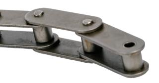
**Double Pitch Straight Sidebar Roller Chains** provide an economical material handling solution for low to moderate loads and distanced sprockets. The prefix "C" and adding 2000 to the ANSI standard number indicates these chains. For pitches 1.5 inches and longer, heavy side plates are noted with the suffix "H." For example, ANSI 60 Double Pitch straight sidebar chain is designated C2060H.
