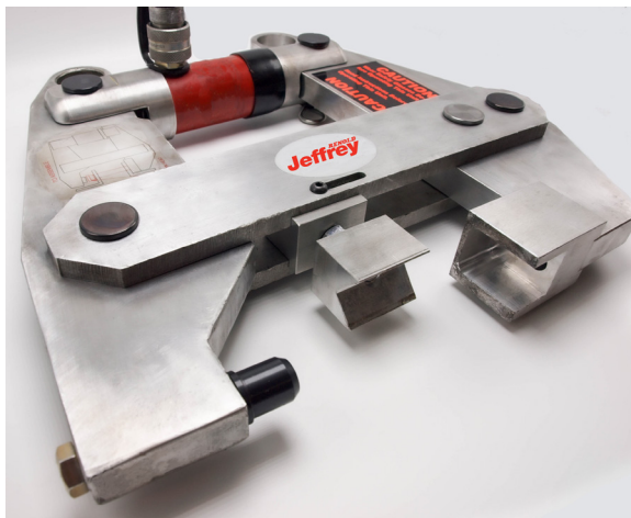
Figure 6. Renold Jeffrey's engineered chain breaker and assembly tool.
