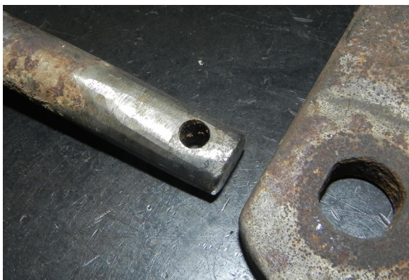
Figure 3. This pin was ground down to make the assembly process easier.
