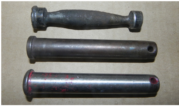
Figure 1. Pins can wear at varying rates. The topmost one is a carbon steel pin that was mistakenly assembled in a stainless steel chain.
