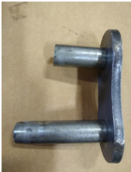
Figure 5. Chain components that were bent during the assembly process and caused the pin to shear.
