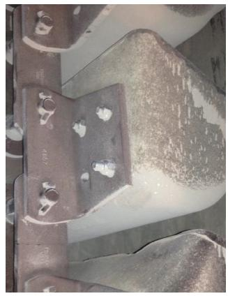
Note the deformity on the bottom bucket in this image. Keep an eye on these signs for warning of more serious and costly issues.
