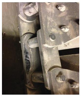
This chain was damaged on the inside link due to misalignment.
