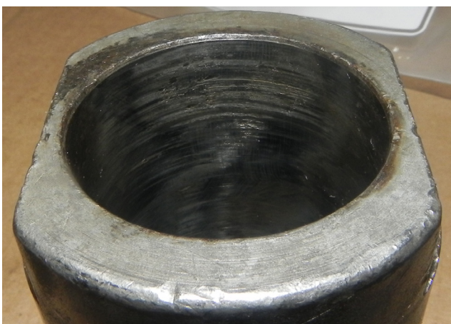
Figure 8. Localised galling on the ID of the chain bushing on the head side of the chain.
