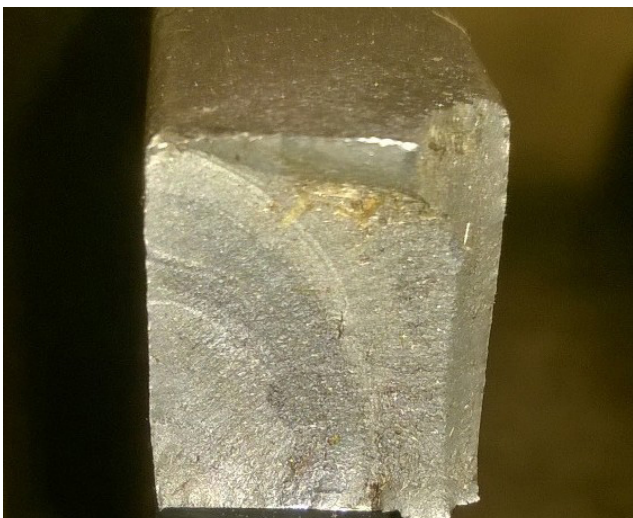
Figure 4. Evidence of long cycle fatigue followed by a fast fracture observed on the fracture surface of the head end sidebar.
