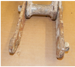
Figure 10. Pin broken even with the sidebars in the shear zone area.
