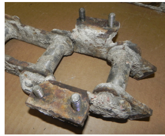
Figure 11. Material from the application covering the outer surfaces of the chain.
