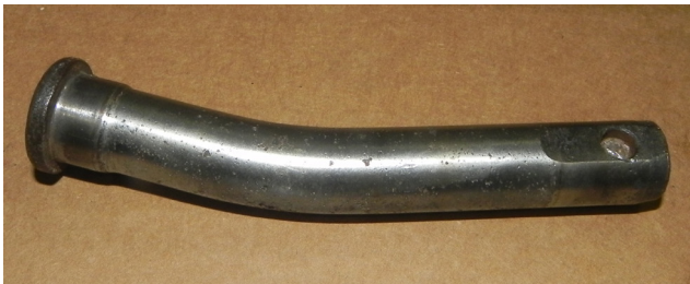
Figure 14. Typical condition of the pins tested showing sufficient ductility.
