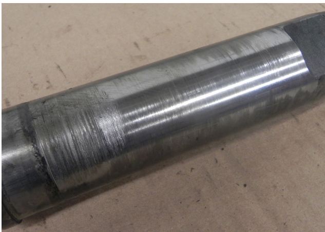
Figure 7. Localised galling on the head side of the pin was present on the bearing surface.
