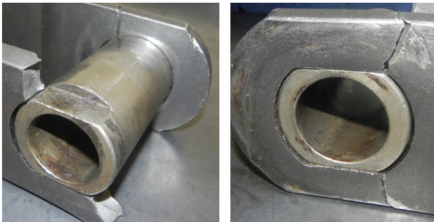
Figure 2. Fractured area on the head end offset bar (left); fractured area on the cotter end offset bar (right).
