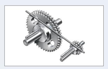
Use a straightedge across the machined faces of the sprockets in several different positions, if possible, as a check against wobble. A nylon or similar line is a good substitute for a straightedge, particularly on longer center distances.
